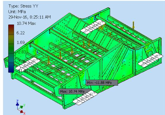
Fig.4. The maximum stress in the structure ( $\sigma_y$ )
