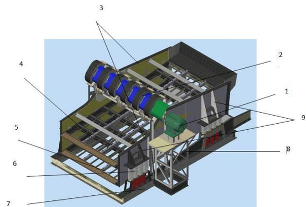
Fig.1 Model of vibrating screen machine
