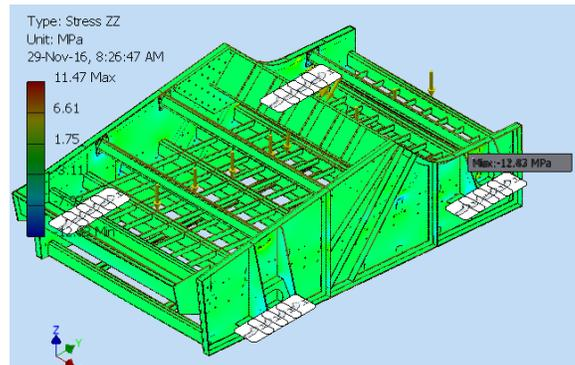
Fig.5. The maximum stress in the structure ( $\sigma_z$ )
