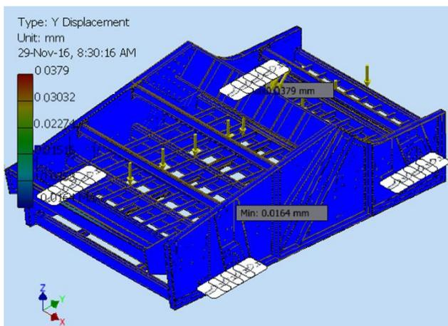
Fig.8. The maximum displacement in the structure (y-y)
