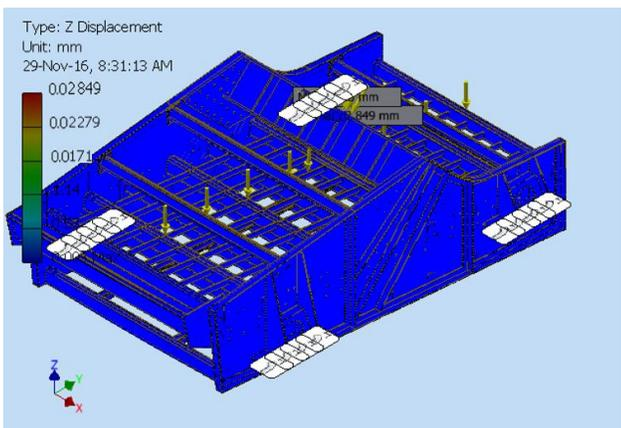
Fig.9. The maximum displacement in the structure (z-z)
