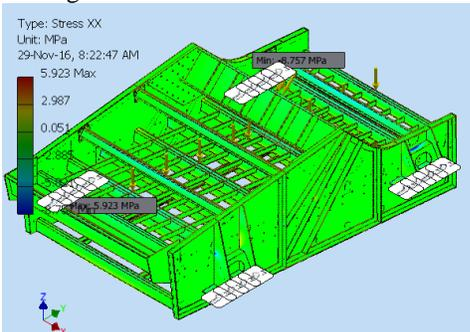
Fig.3. The maximum stress in the structure ( $\sigma_x$ )
