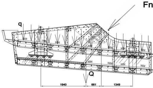
Fig.2. Loads acting on the vibrating screen machine structure
