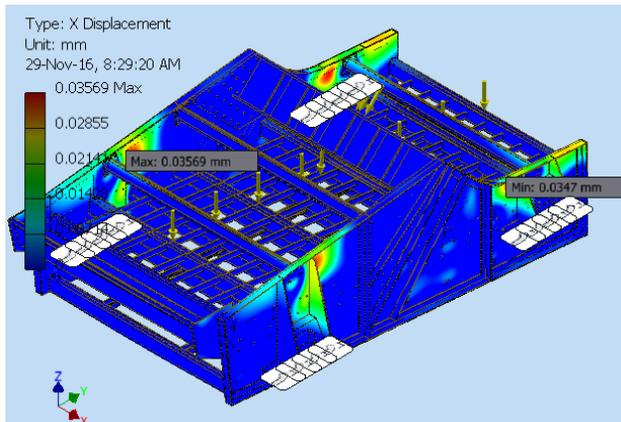
Fig.7. The maximum displacement in the structure (x-x)
