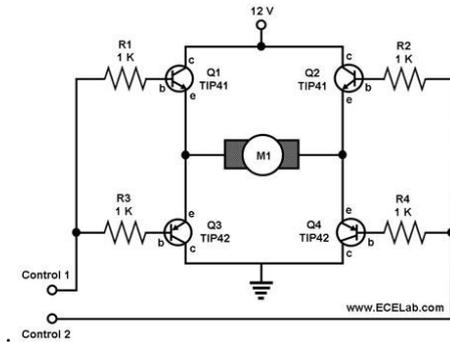
To make the motor go forwards, Q4 is turned on, and Q1 has the PWM signal applied to it. Meanwhile, to make the motor go backwards, Q3 is turned on, and Q2 has the PWM signal applied to it.
