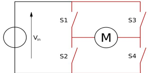
An H bridge is built with four switches (solid-state or mechanical). When the switches S1 and S4 (according to the first figure) are closed (and S2 and S3 are open) a positive voltage will be applied across the motor. By opening S1 and S4 switches and closing S2 and S3 switches, this voltage is reversed, allowing reverse operation of the motor.
