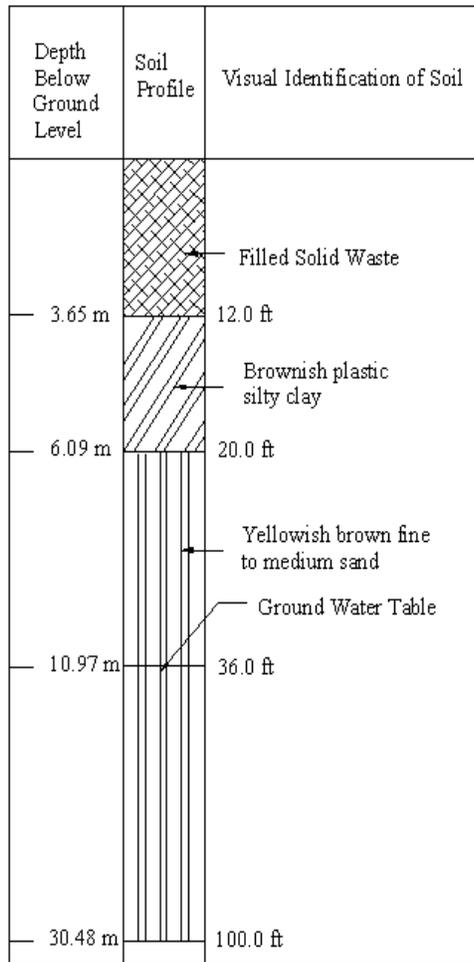
Fig. 5.1 Typical profile of Bore well B1
