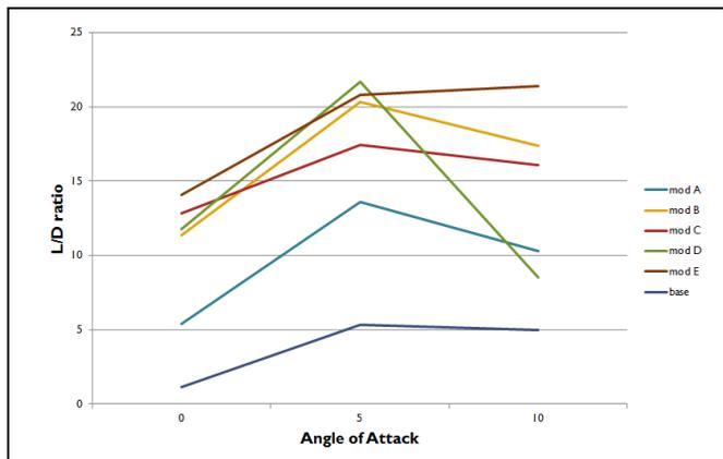
Graph3.5: lift to drag ratio coefficient Vs angle of attack of cylinder model
