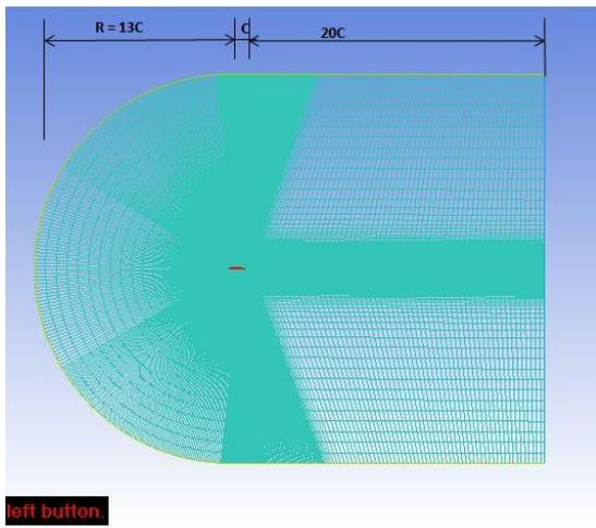
Figure 2.2: Single element airfoil domain size and clustering
