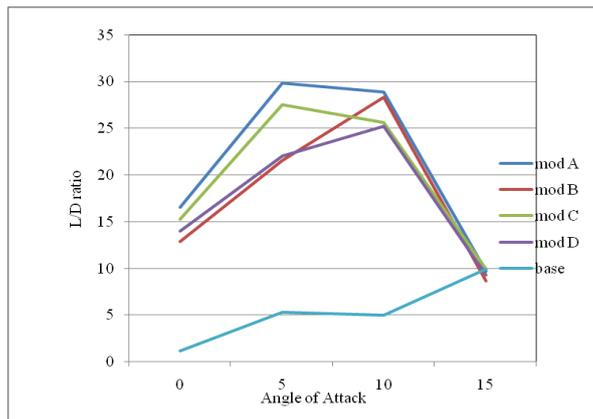
Graph 3.3: Lift-to-drag ratio VS angle of attack
