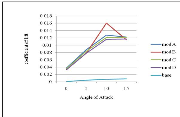
Graph 3.1: Dimples section lift coefficients at 0.3 Mach speed
