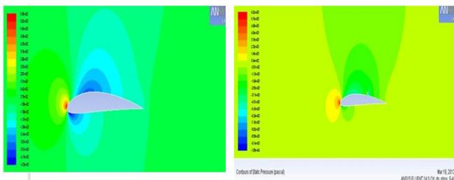
Figure 3.7 : static pressure contours of base 0°Vs cylinder model E at angle of attack 0°
