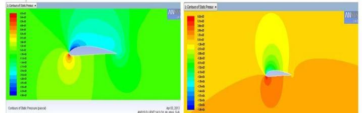
Figure 3.4: Static pressure contours of model A at angle of attack 10<sup>0</sup> degrees Vs base model at 10<sup>0</sup>
