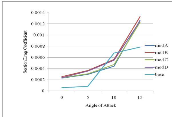
Graph3.2: Sections drag coefficients VS angle of attack
