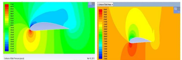
Figure3.5: Static pressure contours of model A at angle of attack 15<sup>0</sup> degrees Vs base model at 15<sup>0</sup>
