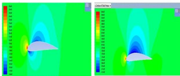
Figure 3.2: Static pressure contours of model A at AOA 0 degrees Vs base model at 0<sup>0</sup>
