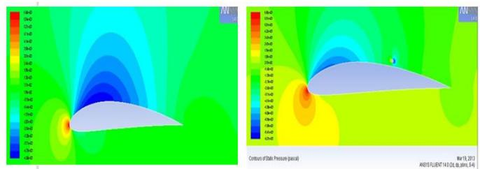
Figure 3.8: static pressure contours of base 5°Vs cylinder model E at angle of attack 5°
