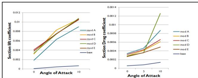
Graph3.4: Section lift and drag coefficient Vs angle of attack of cylinder model
