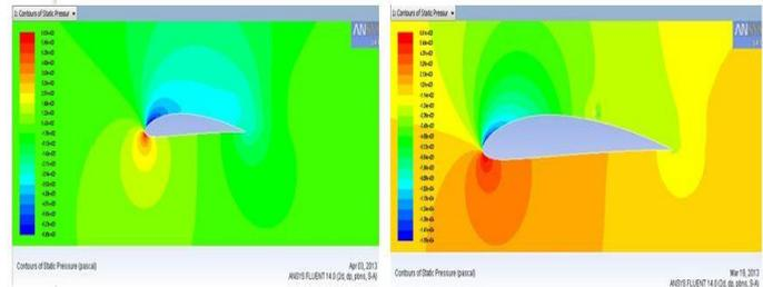
Figure 3.9: static pressure: contours of base 10°Vs cylinder model E at angle of attack 10°
