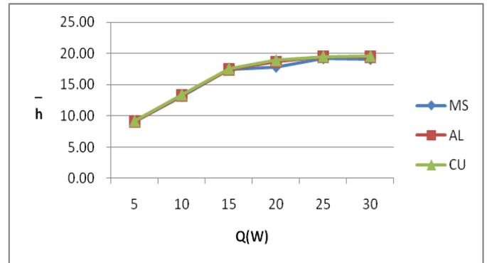
**Graph No. 4.3: Variation of heat transfer coefficient with Heat input for single perforated mild steel, aluminum, copper material respectively**
