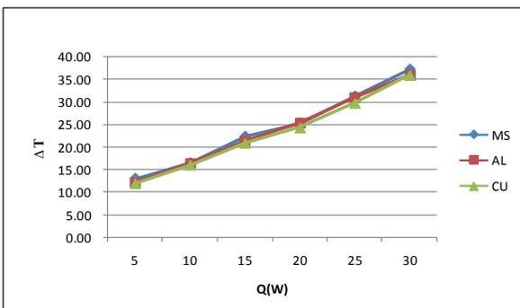
**Graph No. 4.8: Variation of temperature difference with heat input for triple perforated mild steel, aluminum, copper material**
