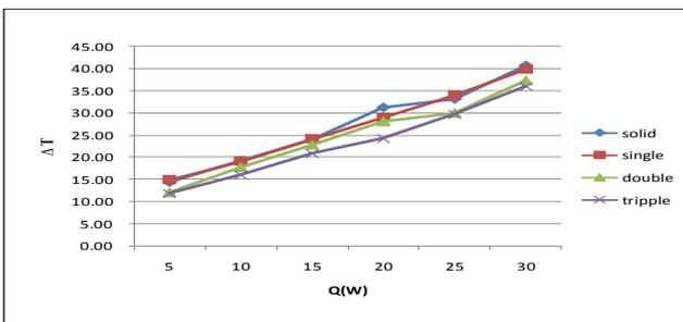
**Graph No. 4.14: Variation of temperature difference with heat input for copper material**
