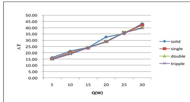
**Graph No. 4.10: Variation of temperature difference with heat input for mild steel**
