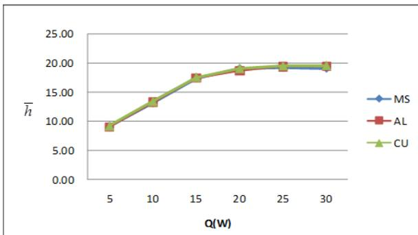
**Graph No. 4.1: Variation of heat transfer coefficient with Heat input for mild steel, aluminum, copper material respectively.**
