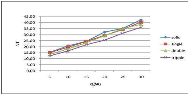
**Graph No. 4.12: Variation of temperature difference with heat input for aluminum material**
