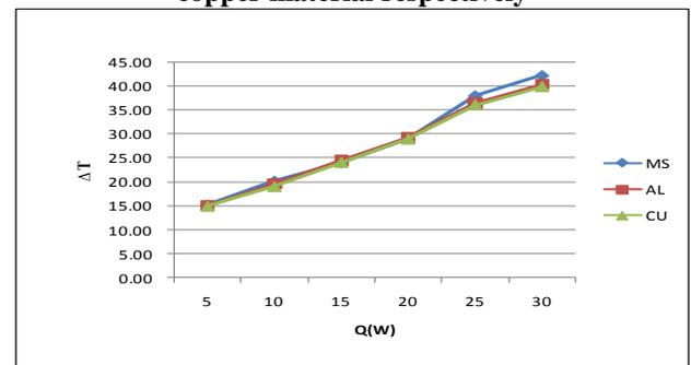
**Graph No. 4.4: Variation of temperature difference with heat input for single perforated mild steel, aluminum, copper material resp.**
