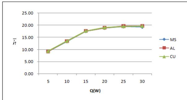
**Graph No. 4.7: Variation of heat transfer coefficient with Heat input for triple perforated mild steel, aluminum, copper material respectively.**
