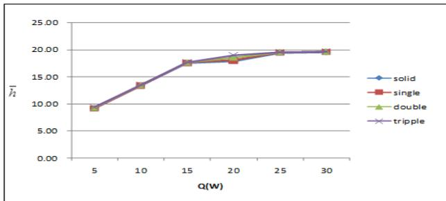
**Graph No. 4.13: Variation of heat transfer coefficient with Heat input for mild steel, aluminum, copper material**
