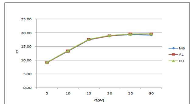
**Graph No. 4.5: Variation of heat transfer coefficient with Heat input for double perforated mild steel, aluminum, copper material respectively.**
