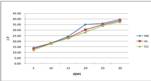
**Graph No. 4.6: Variation of temperature difference with heat input for double perforated- mild steel, aluminum, copper material respectively.**
