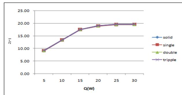
**Graph No. 4.11: Variation of heat transfer coefficient with Heat input for aluminum material**
