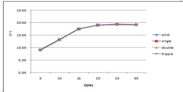
**Graph No. 4.9: Variation of heat transfer coefficient with Heat input for mild steel**
