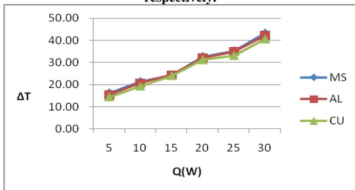
**Graph No. 4.2: Variation of temperature difference with heat input for mild steel, aluminum, copper material respectively.**
