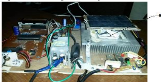
Figure No 2.1B:- Experimental Set up with using thermoelectric cooling 6-Peltier Module (cooler)
