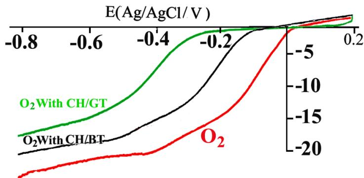
**Figure 7:** Voltammograms of  $\text{O}_2$  in the absence and the presence of the complexes, at Platinum Rotating disk ( $\phi = 2 \text{ mm}$ ,  $\omega = 1000 \text{ rev min}^{-1}$ ), in acetate buffer solution ( $pH = 4.00$ ).
