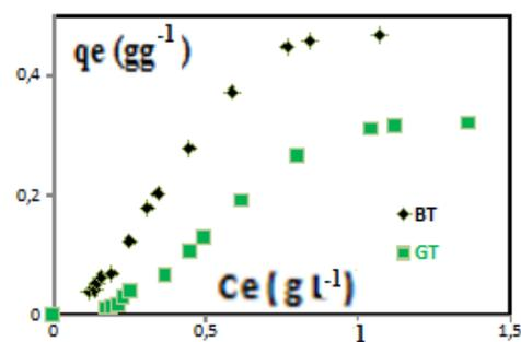
**Figure. 3:** Isotherm equilibrium of GT and BT adsorption into CH at  $T=30^\circ\text{C}$  (pH= 4,  $C_0 = 2 \text{ g dm}^{-3}$  and 0.1 g of CH).
