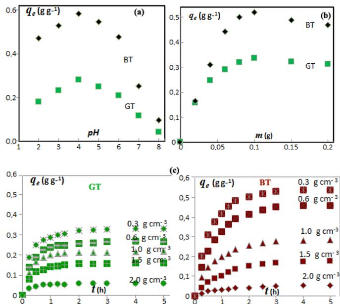
**Figure.2.:** Effects of the experimental conditions on the efficiency of GT and BT adsorption into CH at  $T=30^\circ\text{C}$ , (a) the pH of the tea extracts ( $C_0 = 2 \text{ g dm}^{-3}$ , 0.1 g of chitosan), (b) the chitosan dose (pH=4,  $C_0 = 2 \text{ g dm}^{-3}$ ) and (c) the initial concentration of tea extracts (pH=4, 0.1 g of CH).
