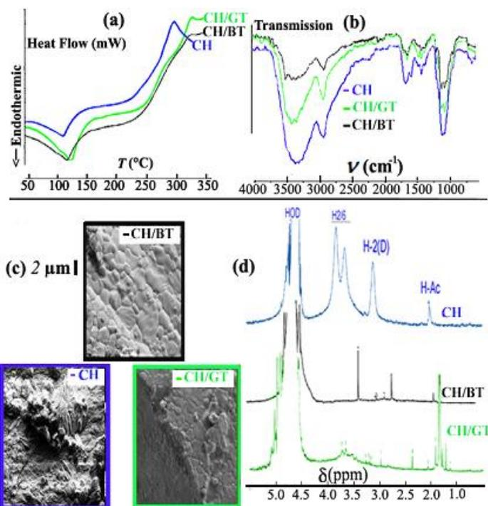
**Figure 4:** (a) DSC thermograms, (b) FTIR spectra, (c) scanning electron micrographs and (d) <sup>1</sup>H NMR spectra of CH and its complexes (CH /GT and CH /BT).
