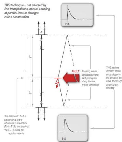
Figure 1- Double Line Travelling Wave Technique
