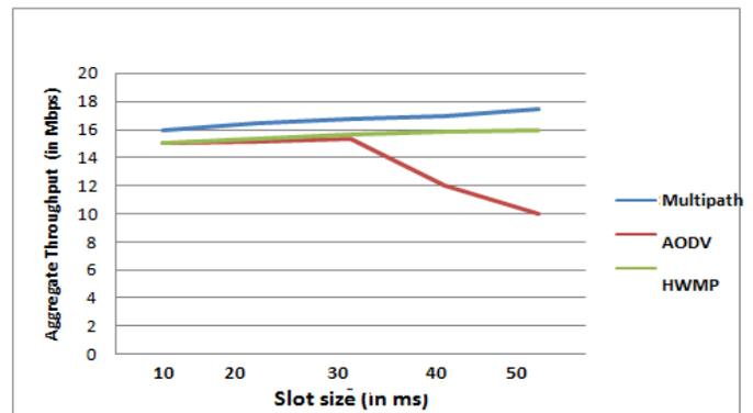
Figure 4 (a) Average Throughput vs. slot size for 100 nodes
