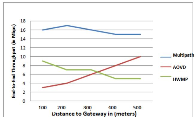
Figure 2 (b) End-to-End Throughput vs. Distance to Gateway
