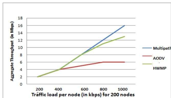
Figure 3 (b) Average Throughput vs. Traffic node (in kbps) for 200 nodes
