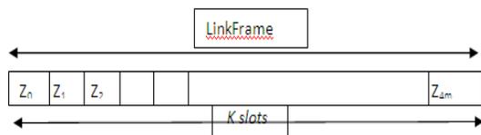
Figure 1. Frame Structure of Link Frame
