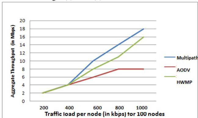
Figure 3 (a) Average Throughput vs. Traffic node (in kbps) for 100 nodes
