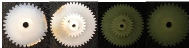
Figure 1: Defective gears(a,b) Non defective gears(c,d)
