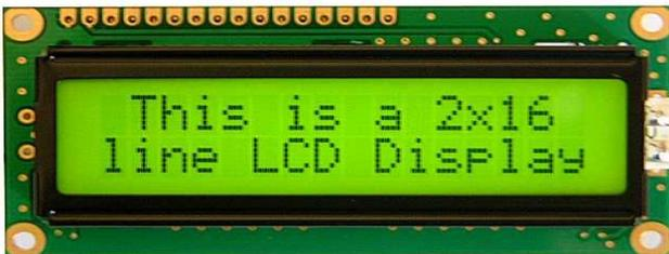
Figure (6): 2X16 LCD Module
