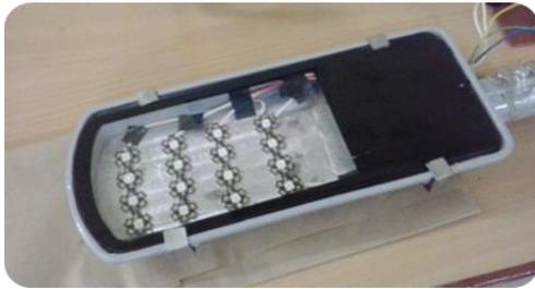
Figure (5): Encapsulated LED Lamp
