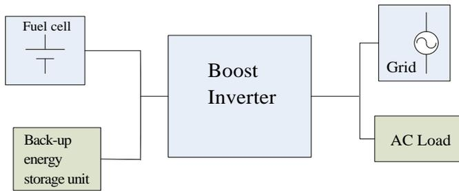
Fig.4 Block diagram for the proposed grid connected fuel cell system
