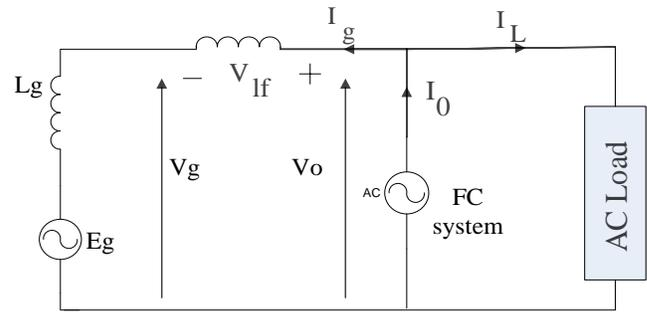
Fig.2 Equivalent circuit of grid connected FC system
