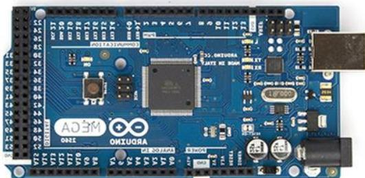
Figure 2: Arduino Mega 2560
