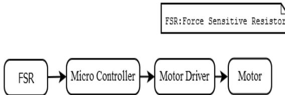
Figure 3: Block diagram
