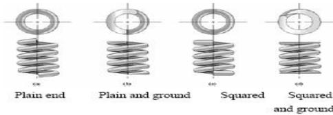
(Fig.2.2 Compression helical spring)
