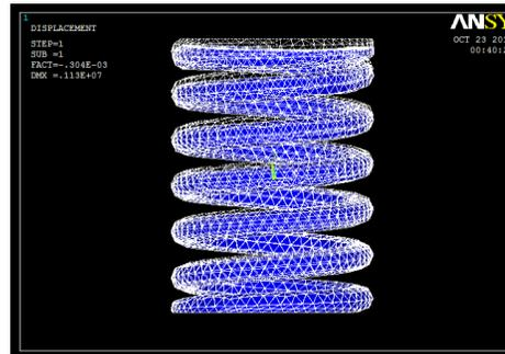
(Fig 3.3 Buckling Analysis of Chrome Vanadium)
