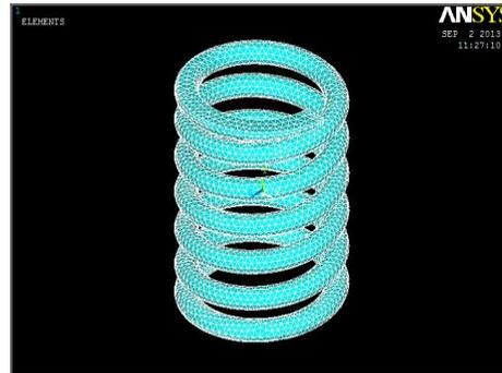
(Fig 3.2 Mesh of Primary Suspension Spring)
