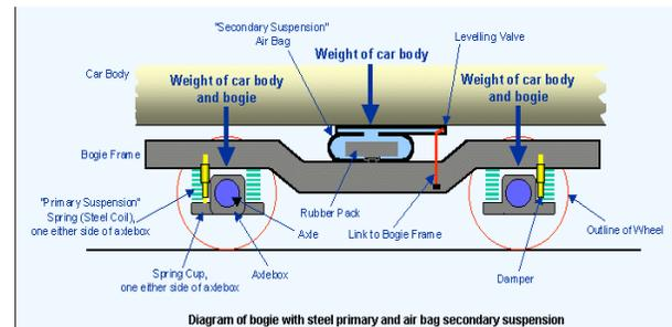
(Fig 1.2 Primary Suspension System)
