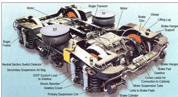
(Fig 1.1 Different Bogie Parts)
