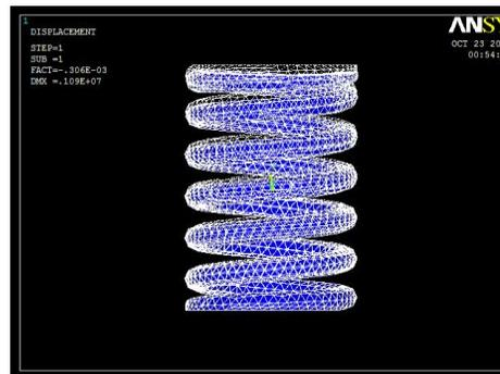
(Fig 3.4 Buckling Analysis of 20NiCrMo<sub>2</sub>)
