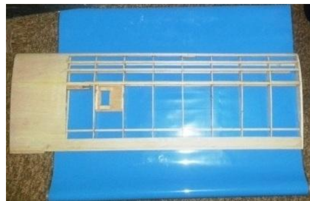
Fig 2: Lamination of Clark Y Airfoil
