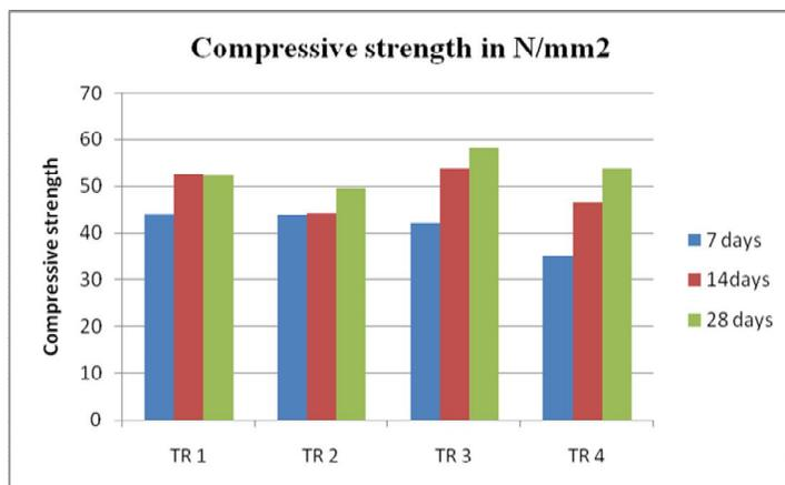
**Figure 2 Compressive strength comparison for trial mixes**
