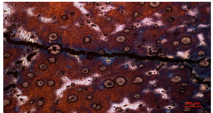
Fig.4. crack near the quenching organization (100X has been corroded)
