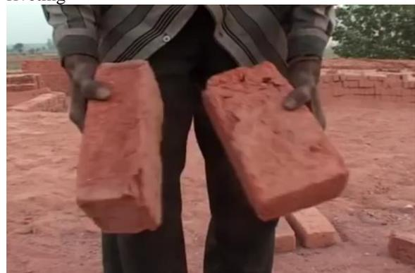
**Fig.6-** Snapshot of a video showing ringing sound of a brick
