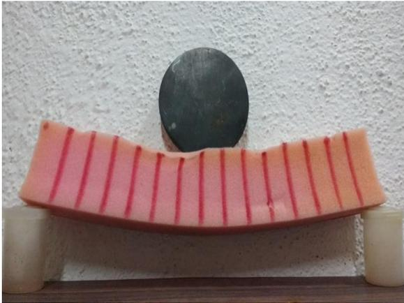
**Fig.2-** Use of physical models to understand forces in a beam
