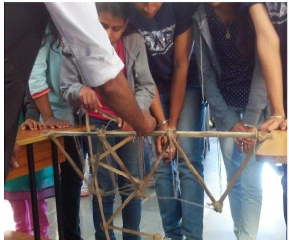
**Fig.1-** Use of physical models to understand forces in a truss
