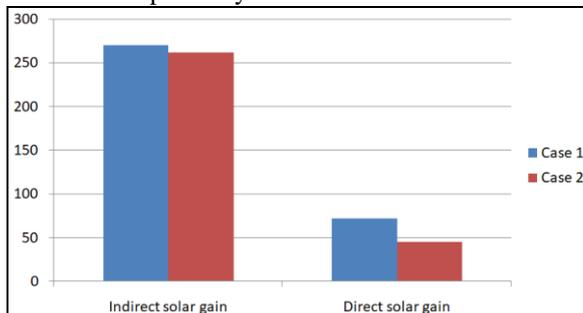
Graph 1 Indirect and direct solar gain comparison
