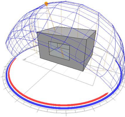
Figure 3 Room model with window on South facade in Ecotect software
