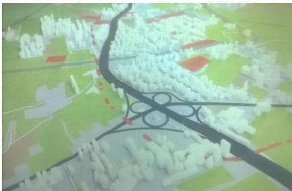
**Fig 5. Proposed Cloverleaf arrangement at Chakan Chowk**
