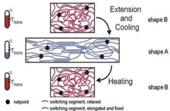
Figure 3 c: Shape memory polymer with molecular network & switch points
