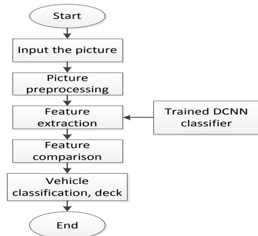
Fig 1: Block diagram of vehicle image comparison
