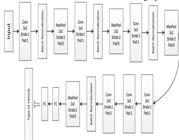
Fig 2: The CNN network structure
