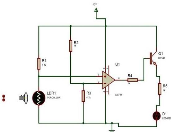
Figure: 6 Automatic ON-OFF control circuit diagram
