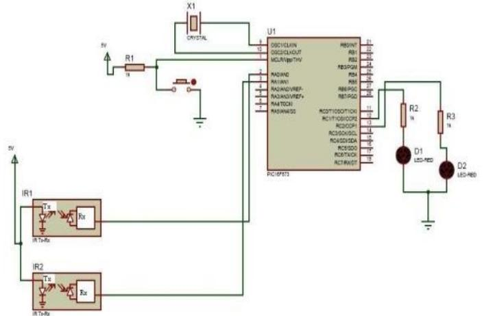
Figure: 8 Light controller circuit diagram using microcontroller
