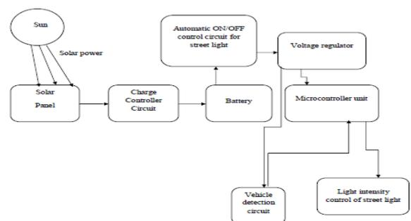
Figure: 4 Solar Powered Vehicle Detect Auto Intensity Controlled
