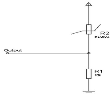
Figure: 3 CdS photocell circuit
