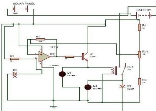
Figure: 5 Charge controller circuit diagram
