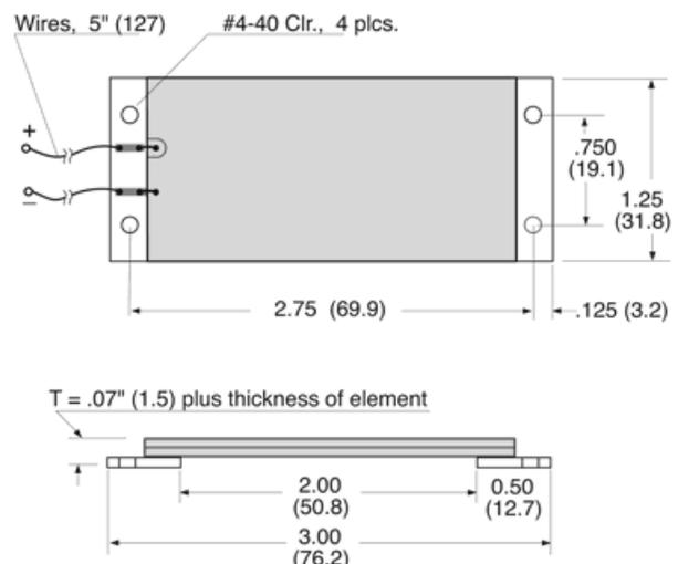
Figure 2, Peizo energy harvesting generator – Double quick mount dimentions- 503 size
