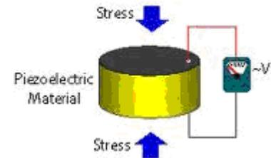
Figure 1. Piezoelectric effect
