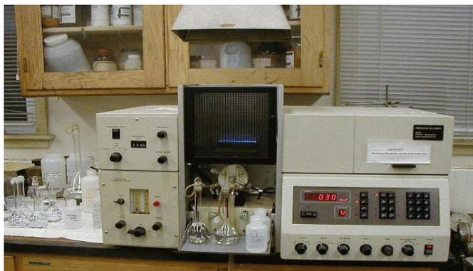
Figure 1:- Atomic Absorption Spectrometer
