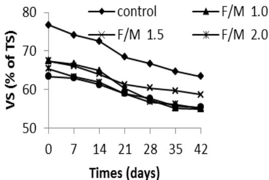
Fig. 1 The VS reduction during the period of anaerobic digestion with different I/S ratio
