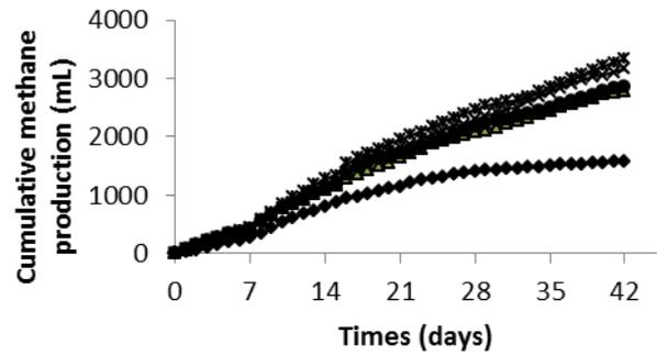
Fig. 2. The methane yield in the anaerobic digestion different I/S ratios
