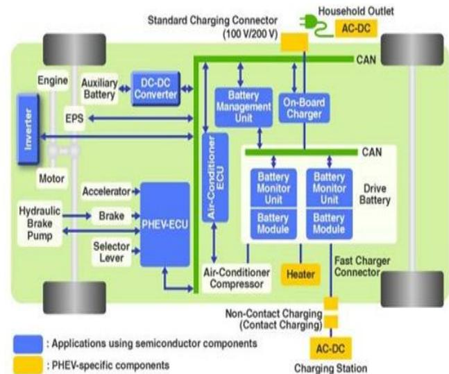
Fig 1: Block Diagram of Plug In Hybrid Electric Vehicle
