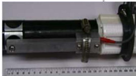
(a) Transducer for handle force measurement
