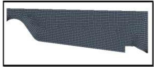
Fig. 2. Meshing pattern of the model
