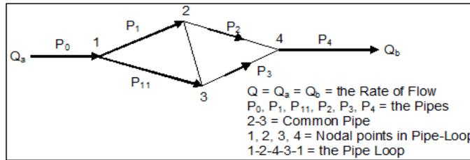
Figure 1: Plan of A Pipe Network (with continuity consideration)
