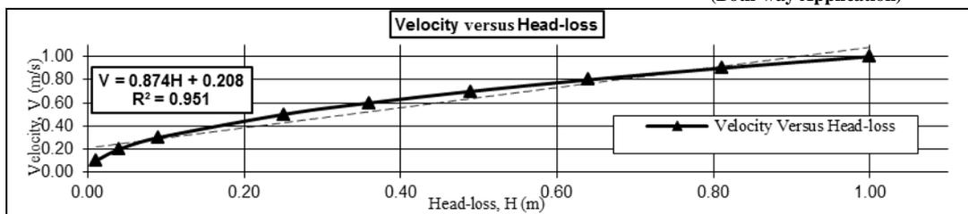
Figure 5: Profile Of The Head-Loss With Flow Velocity (V)
