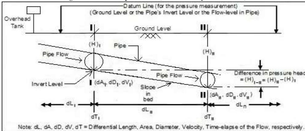
Figure 2: Profile Of Pressure Head & Loss In The Distribution Flow Dynamics
