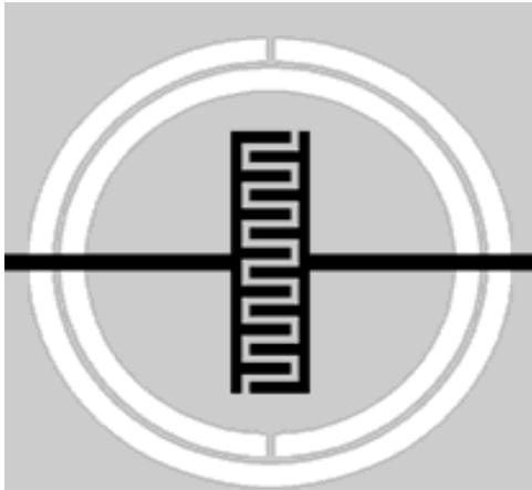
Fig 2. Proposed geometry of compact micro-strip high pass filter
