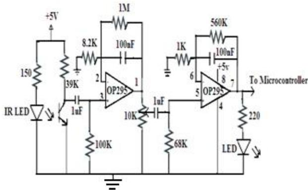
**Figure 5. Signal conditioning circuit for pulse rate measurement**
