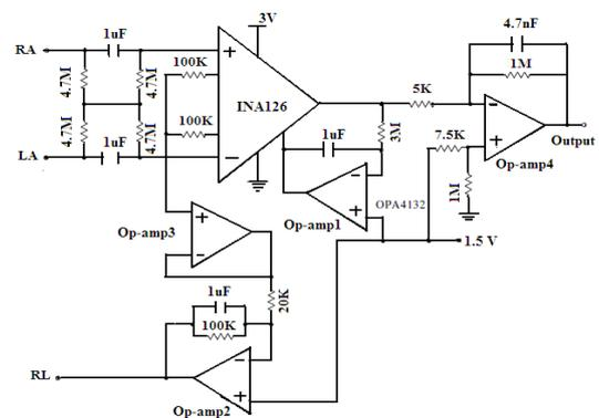
**Figure 4. Signal conditioning circuit for ECG sensor**
