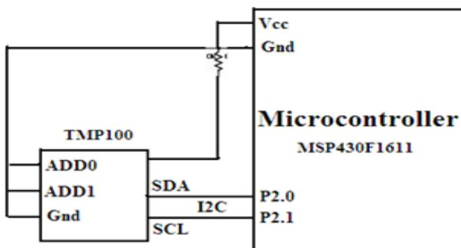
**Figure 6. Simple interfacing of Digital temperature sensor**
