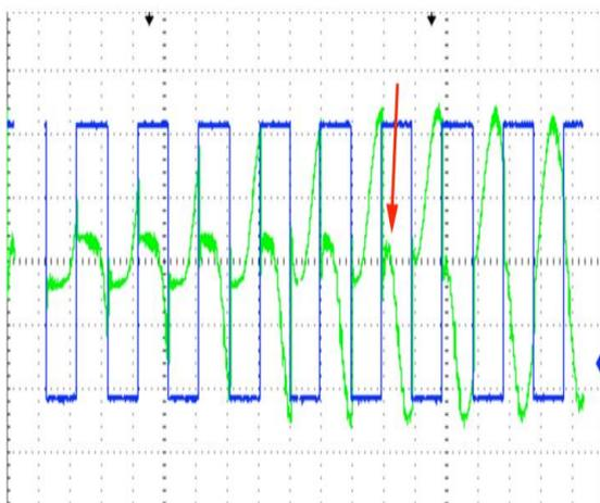
**Figure. 4.6:** Piezo generator vibrating at 2 Hz and SSHI circuit with 1 Hz external control signal slightly off sync. Shows dependence on when the switching is done and that it needs to be a bit after the voltage peak due to reduced phase
