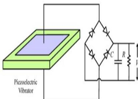
Figure.1: PVH with commonly used rectifying circuit.
