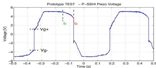
**Figure. 4.2:** P-SSHI piezo voltage with an output load of  $R = 2.7 \text{ M}\Omega$ . The voltage peak is a  $t_1$  and the actual inversion happens a  $t_2$ . The inversion factor is estimated to be  $\gamma = -\frac{V_{g+}}{V_{g-}} = 0.35$ .
