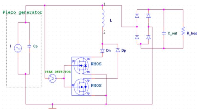
**Figure.3(a):** Simplified PSpice simulation circuit for analyzing the P-SSHI topology.
