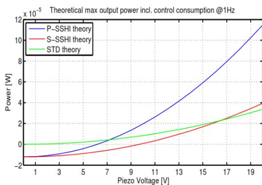
**Figure. 4.7:** Theoretical maximum output power of P-SSHI ( $\gamma = 0.35$ ) and S-SSHI ( $\gamma = 0.21$ ) with the estimated control power consumption subtracted. Compared with the maximum output power of the standard full bridge for vibrations at 1 Hz as a function of the piezo open circuit voltage,  $V_p$ .
