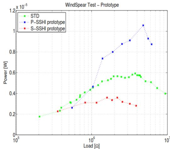
**Figure. 4.7:** Measurement results of the Parallel-SSHI and Series-SSHI prototype along with the standard full bridge, STD.
