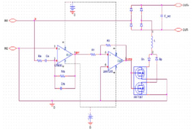
**Figure.3 (b):** Simplified PSpice simulation circuit for analyzing the S-SSHI topology.
