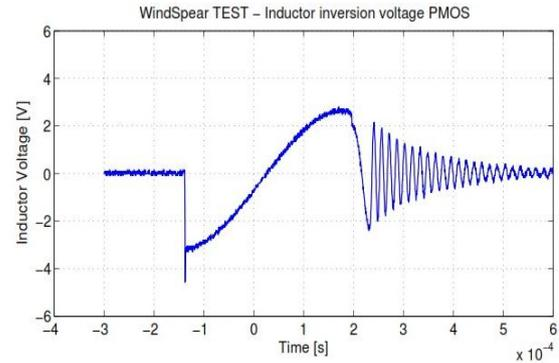
**Figure. 4.3:** P-SSHI inductor inversion voltage when PMOS turns ON. The load connected is  $R=2.7 \text{ M}\Omega$ .
