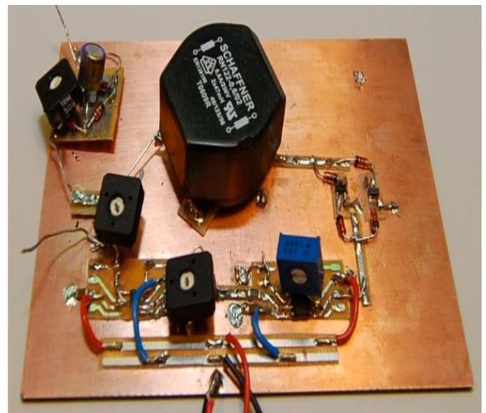
**Figure. 3(C):** Implemented P-SSHI prototype.
