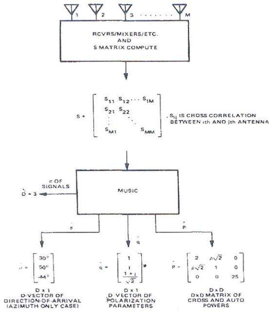
Fig. 2. Block diagram for multiple signal classification.
