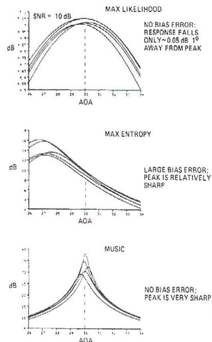
Fig. 4. Example of azimuth-only DF performance (scale expanded about weaker signal at 30°).
