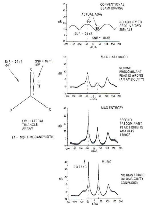
Fig. 3. Example of azimuth-only DF performance.
