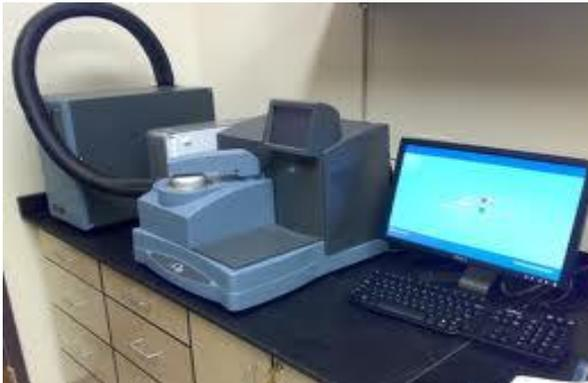
**Fig.2. Differential Scanning Calorimetry**
