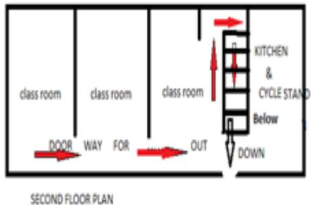
The building plans explain the different room positions and the accommodations, door and stair case location. It explains where the fire started, speeded, the way it was blocked the routes and arrest the movement of the children and the causes the lives losses.
