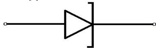
Figure 4: Symbol of Tunnel Diode
