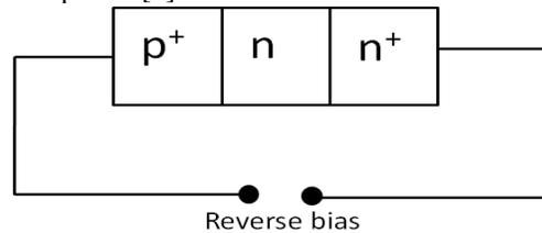
Figure 6: Structure of TRAPATT diode
