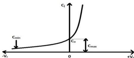
Figure 2 (b): Capacitance variation in Varactor diode with bias
