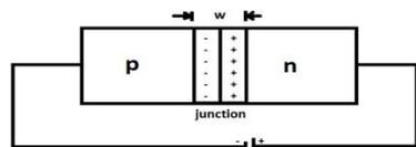
Figure 2 (a): Diagram of Varactor diode
