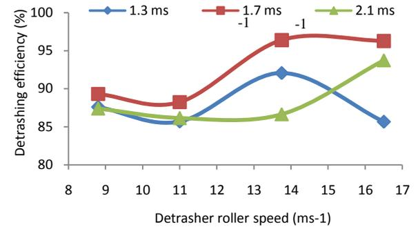
Fig. 5 Sensitivity of de-trashing efficiency and de-trasher roller speed for the different input roller speeds at 0 degree spiral angle
