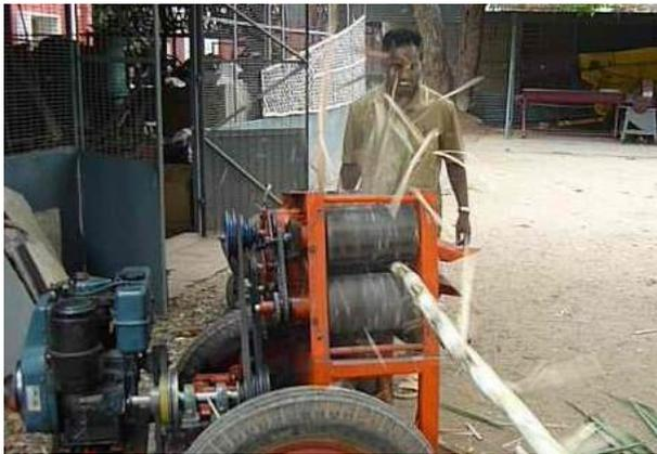
Fig. 3 Test rig for de-trashing studies
