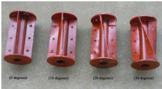
Fig. 2 Different de-trasher rollers
