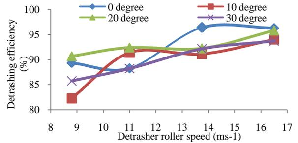
Fig. 4. Variation of de-trashing efficiency with respect to spiral angle of de-trasher brushes and de-trasher brush roller speed
