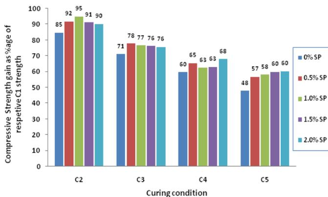
**Figure 3: Compressive Strength gain as %age of respective concrete cured in C-1 due to different SP dosage.**
