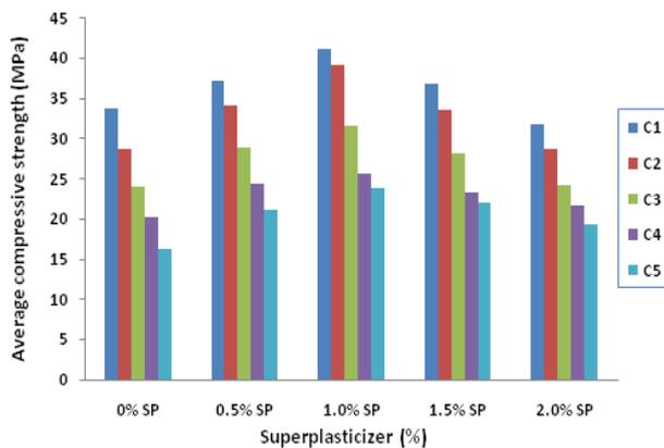
**Figure 2: Effect of superplasticizer on average compressive strength of concrete under different curing conditions.**
