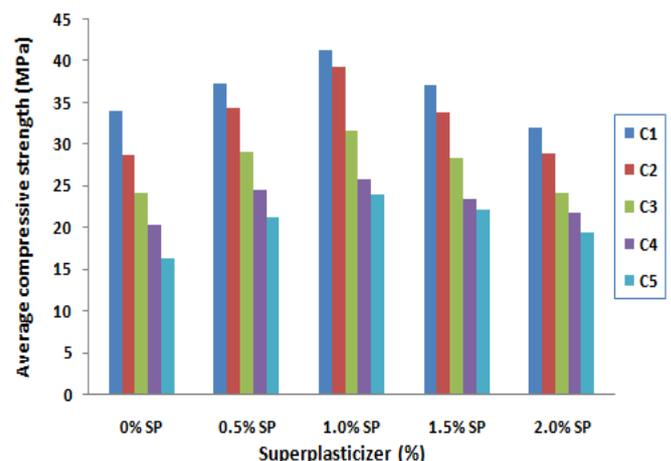
**Figure 1: Effect of curing conditions on average compressive strength of concrete**
