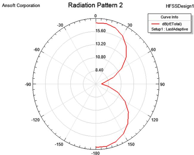
Figure 5: Radiation of Total E-field
