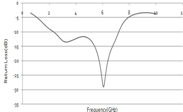
**Figure 2** Return loss of proposed multiband antenna
