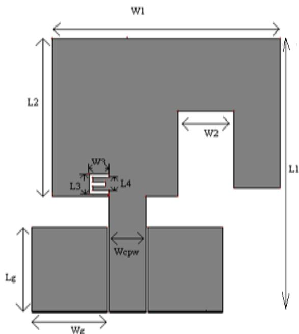
**Figure 1** Geometry of proposed Antenna
