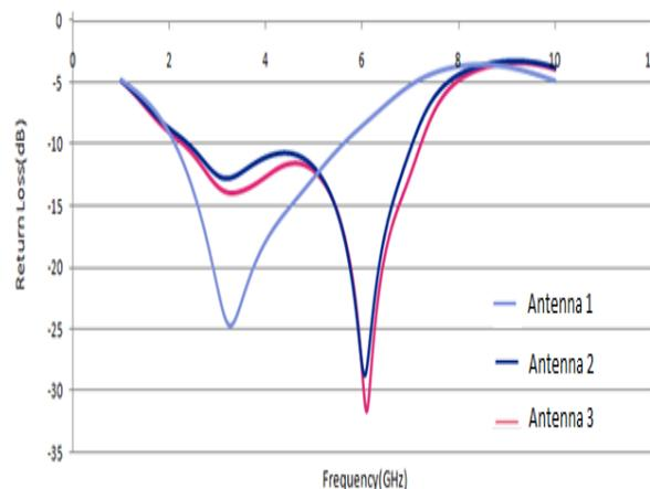
**Figure 3** Return losses of antenna 1, antenna 2, antenna 3
