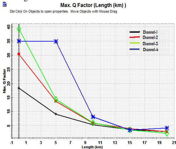
**Fig.6.2 Q Factor vs Lengths of optical fiber**
