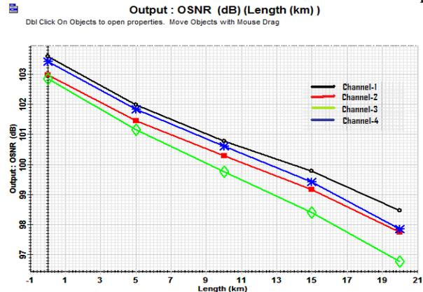
**Fig.6.4 OSNR vs Lengths of optical fiber**
