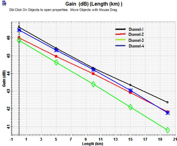
**Fig.6.1 Variation in Gain vs Lengths of optical fiber**
