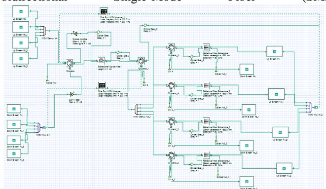
Figure 5.1 Schematic of a bidirectional RoF system
