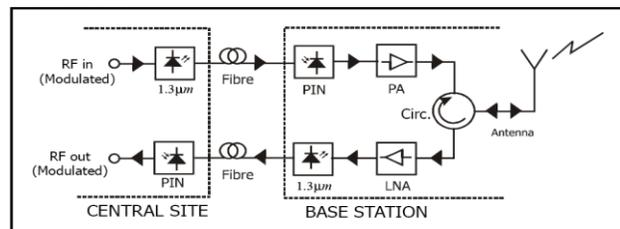
Fig.2. Radio over Fiber System
