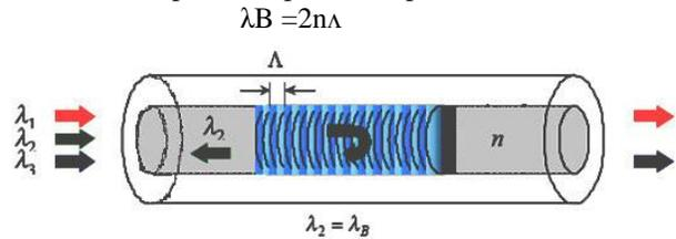
Fig.4.Principal of operation of Fiber Bragg Grating
