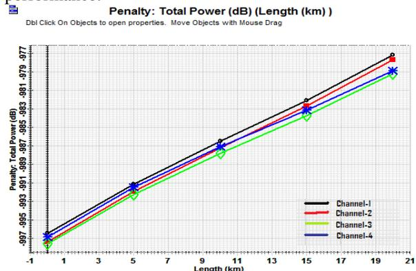
**Fig.6.5 Penalty vs Lengths of optical fiber**
