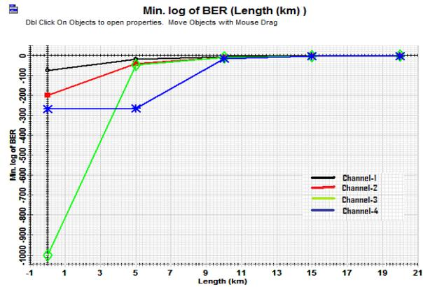
**Fig.6.3 BER vs Lengths of optical fiber**
