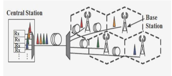
Fig . 1. Scenario for RoF link with photonic down conversion. The base stations (BS) are connected to the central station (CS) through optical fiber.
