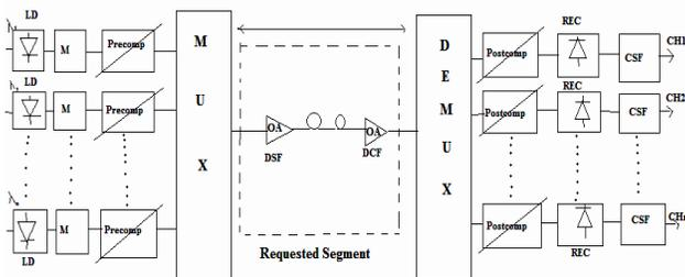
Fig 3.Configuration of typical WDM transmission system.
