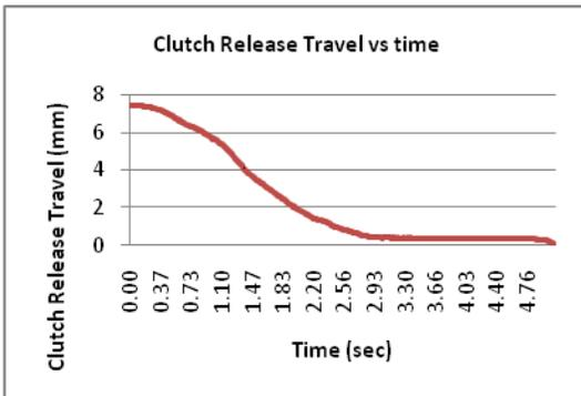
Figure XI: Variation of Clutch Release Bearing Stroke with Time.
