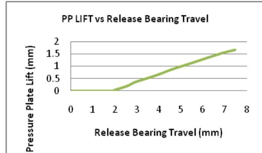
Figure XIV: Variation of Pressure Plate Lift with Release Travel
