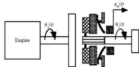
Figure VIII: The displacements in power transmission driveline of an automobile
