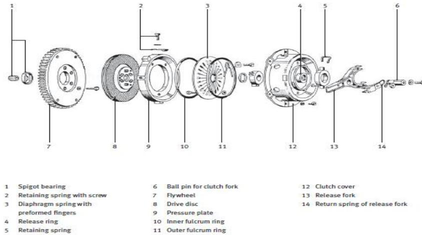
Figure I: Components of Clutch
