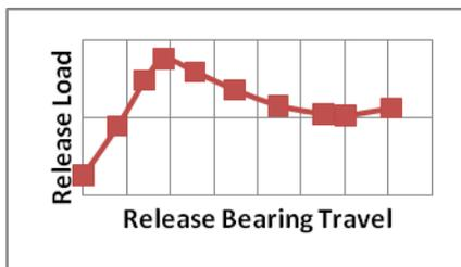
Figure IV: Representation of release load with release bearing travel
