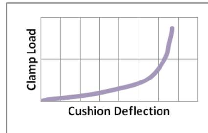
Figure VI: Representation of clamp load with cushion deflection
