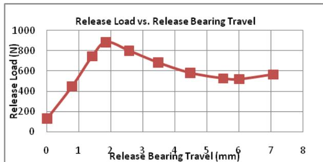
Figure XII: Variation of Release Load with Release Travel
