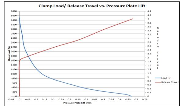
Figure XV: Variation of Clamp Load with Release Travel
