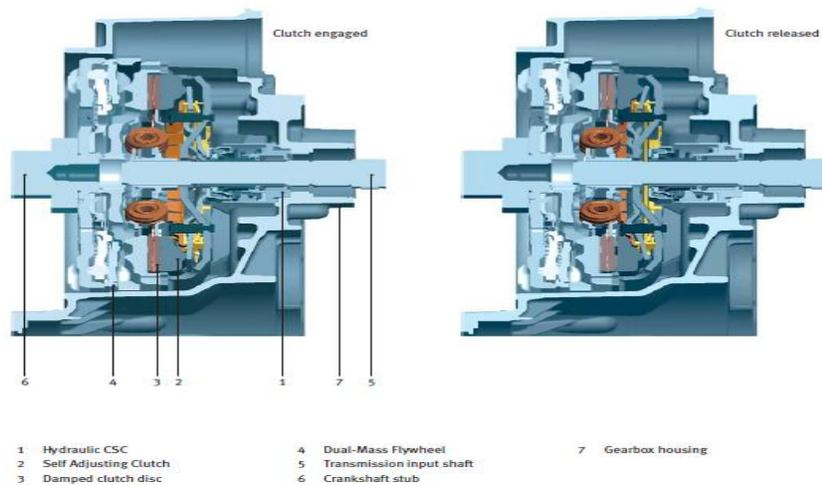
Figure II: Shows the engagement and disengagement of clutch
