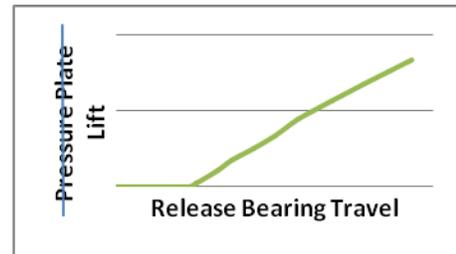
Figure V: Representation of pressure plate lift with release bearing travel
