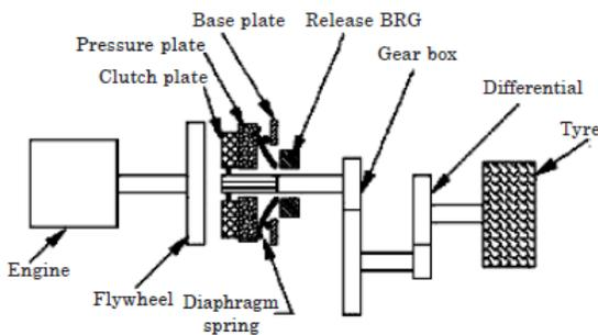
Figure VII: Driveline of an automobile
