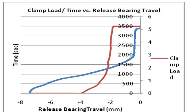
Figure XVI: Variation of Clamp Load and Time with Release Travel
