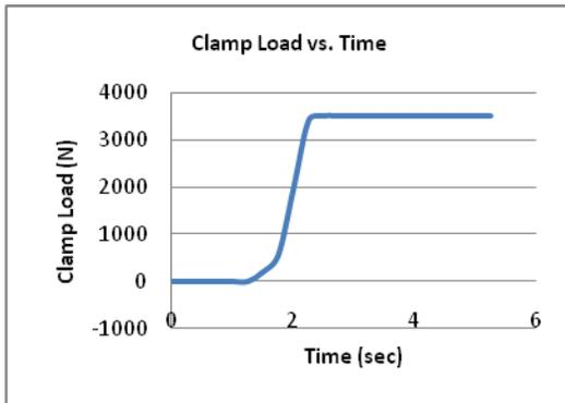
Figure XVII: Development of Clamp Load with Time
