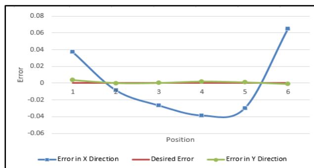
Fig. 5 Error in X and Y Direction for Straight Line Generation Problem
