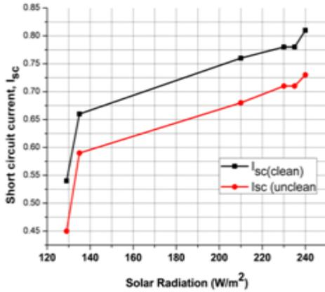
Figure 2 The nature of short circuit current for clean and unclean surface with solar radiation
