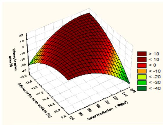
Figure 4 Variation of efficiency for clean and unclean surface with solar radiation.
