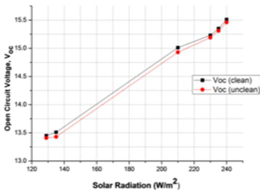
Figure 3 The nature of open circuit voltage for clean and unclean surface with solar radiation
