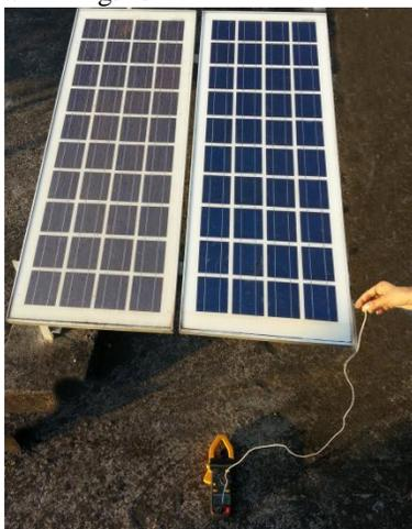
Figure 1. Image of dusty (left) and clean (right) surface.
