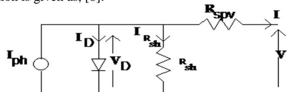
Fig. 1, PV- Cell Equivalent Circuit.
