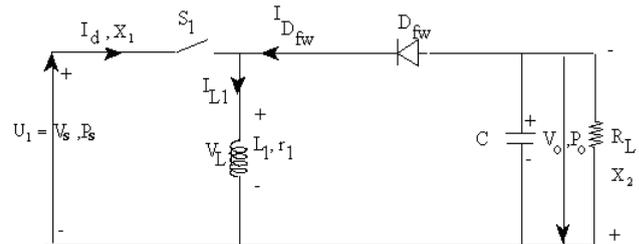
Fig. 5, Switched models for the ideal Buck-Boost converter.
