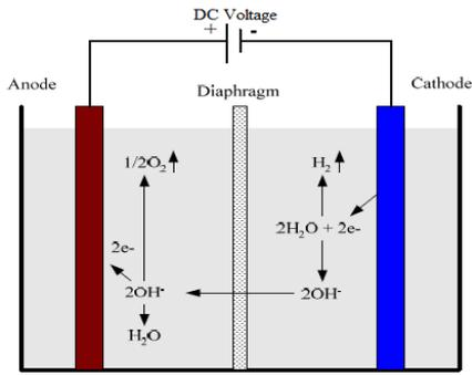
Fig. 6, Schematic diagram of an alkaline type Electrolyzer.
