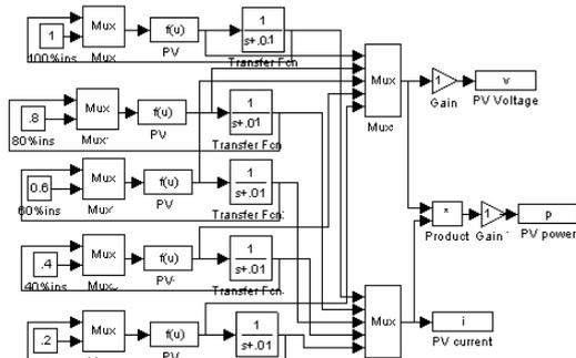
Fig. 2, PV array Matlab/Simulink model for varying Insolation
