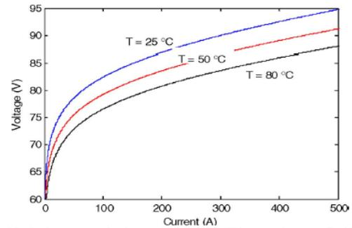
Fig. 7, *V-I* characteristics of the H<sub>2</sub>-Electrolyzer Cell model under different temperatures.
