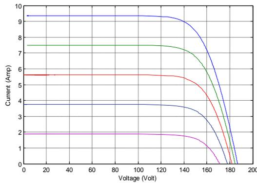
Fig. 3, V-I-P Relations between voltage, current and power of the PV array at different Insolation.
