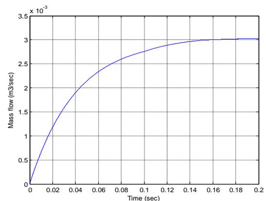
Fig. 15, Output of hydrogen flow from Electrolyser
