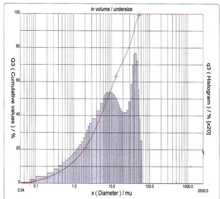
Fig. 1. Particle size distribution of iron ore tailings
