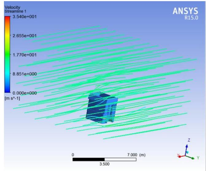
Figure 4: Velocity streamline plot for the original truck model
