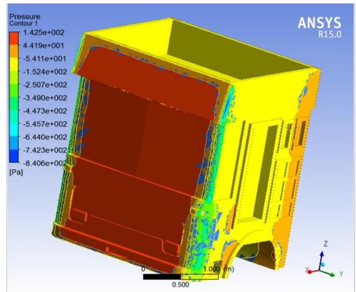
Figure 5: Pressure distribution plot for original truck model
