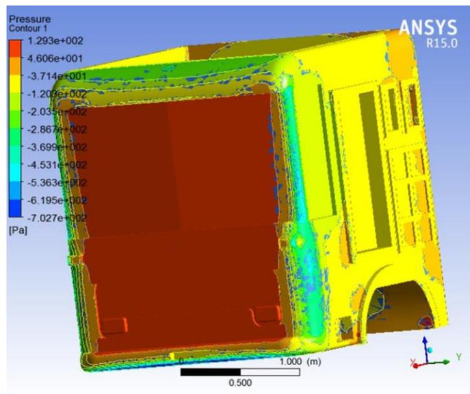
Figure 7: Pressure distribution plot for the modified truck model
