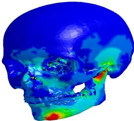
Figure 5: vonMises stresses at 3ms
