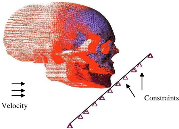
Figure 4: Load and boundary conditions
