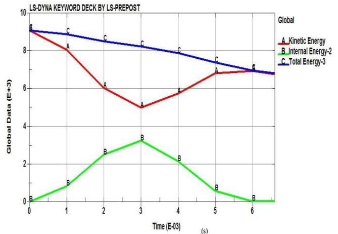
Figure 7: Energy plot with respect to time
