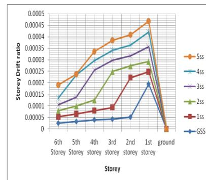
Fig. 3(a): Storey drift and soft storey position (Zone-I)
