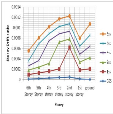
Fig. 3(b): Storey drift and soft storey position (Zone-II)
