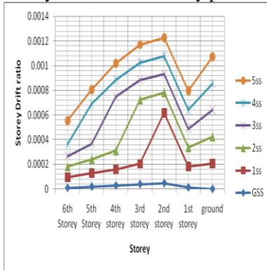
Fig. 3(c): Storey drift and soft storey position (Zone-III)
