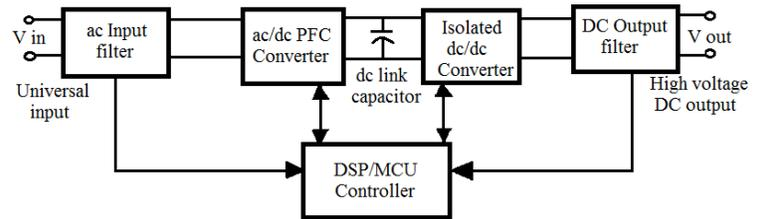
Fig. 1. Simplified system block diagram of a Universal battery charger.
