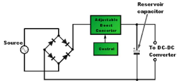
Fig. 3. A Typical PFC Circuit
